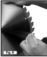
2. Remove the blade from the saw and clean pitch build-up from the blade (Fig. K) Pitch build-up can block the laser and prevent it from accurately indicating the line-of-cut.
